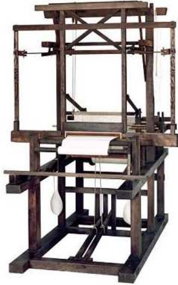
Sakichi's first invention: The Toyoda wooden hand loom
