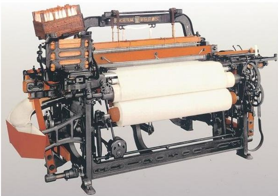
The Type G automatic loom
